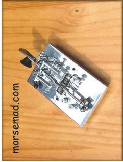
090 .....American McElroy bug, "Hole In The Wall" Made by Telegraph Apparatus Co. Circa 1936/1938. TAC - a company involving T.R. McElroy, this key features a square main frame with a large circular hole through the centre, thus acquiring the name the Hole In The Wall.
