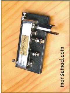
084..... Australian Jigger Bug. Here is another great Australian Simplex Auto Standard Model semi automatic key with a black base. The brass label reads "THE SIMPLEX AUTO (REGD) MANUFACTURED BY LEO G. COHEN MELBOURNE VIC". Melbourne telegraphist Leo Cohen stopped making Simplex Auto jiggers after he went into the Army on 13th Nov. 1939, but his name appears on the Simplex Auto labels up to about S/No 5xxx.
